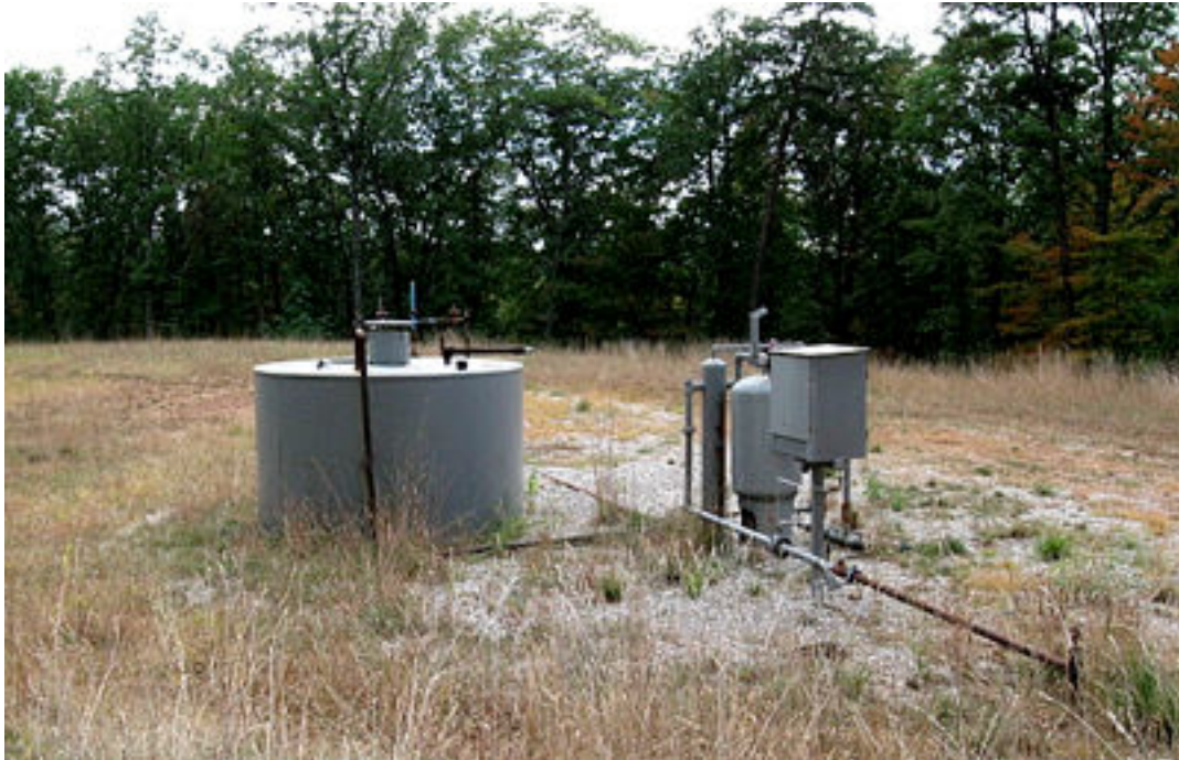
Natural gas well in Putnam county, West Virginia, without required secondary containment for condensate storage tank.
